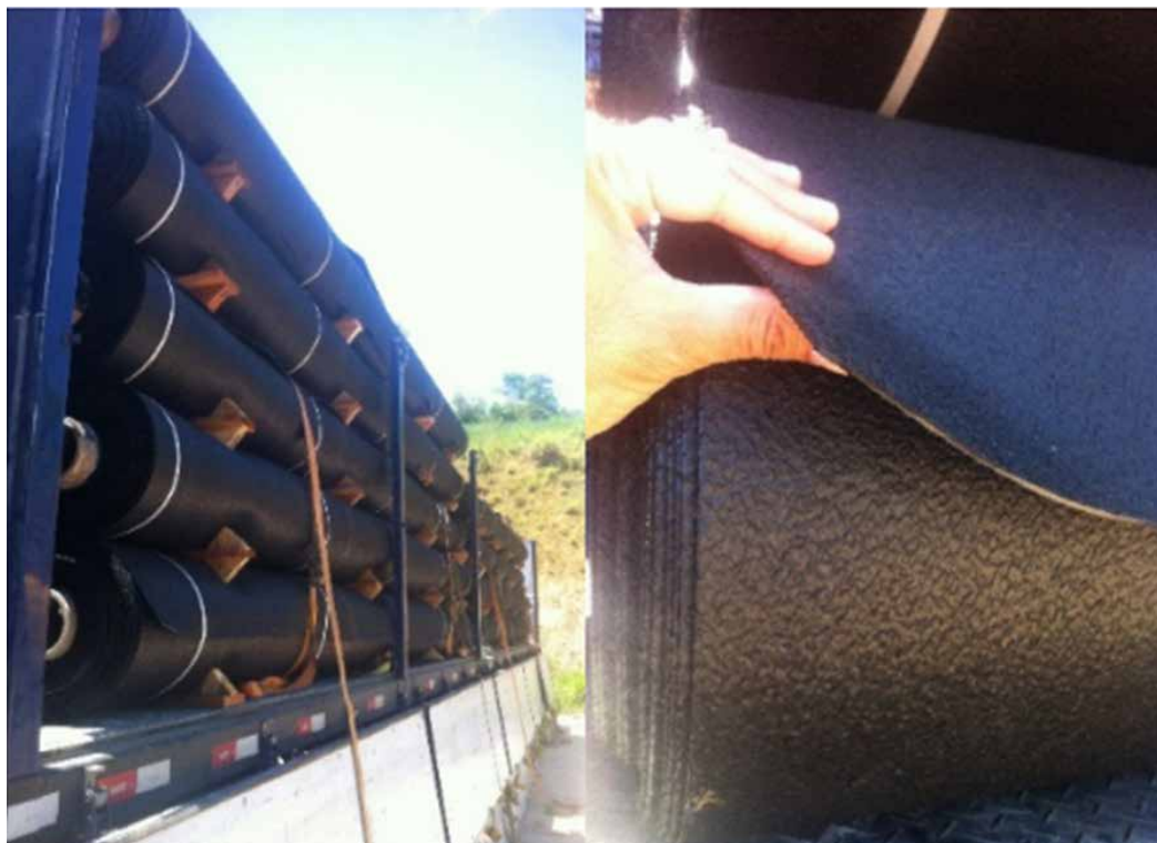
Figura 7: Manta de PEAD – 2,0 mm
