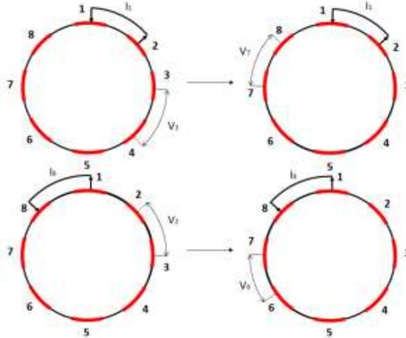
Figure 1. Schematic explaining the adjacent pattern.
