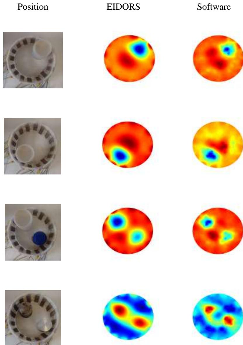
Figure 7. Experimental inhomogeneity estimated.
