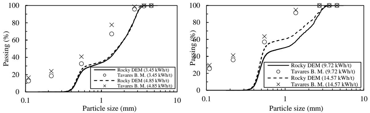
Figure 5 – Comparison between the modelled and simulated progeny size distributions for a single particle impact of particles of 5.47 mm for different impact energies for the copper ore particles.
