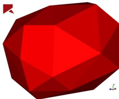
Figure 2 – Generic particle shape of a 5.47 mm particle adopted in the simulations.
