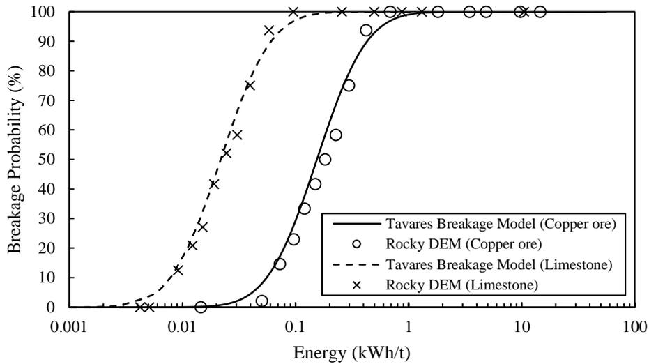
Figure 3 - Comparison between the modelled and simulated breakage probability for a single particle impact of particles of 5.47 mm for different impact energies.
