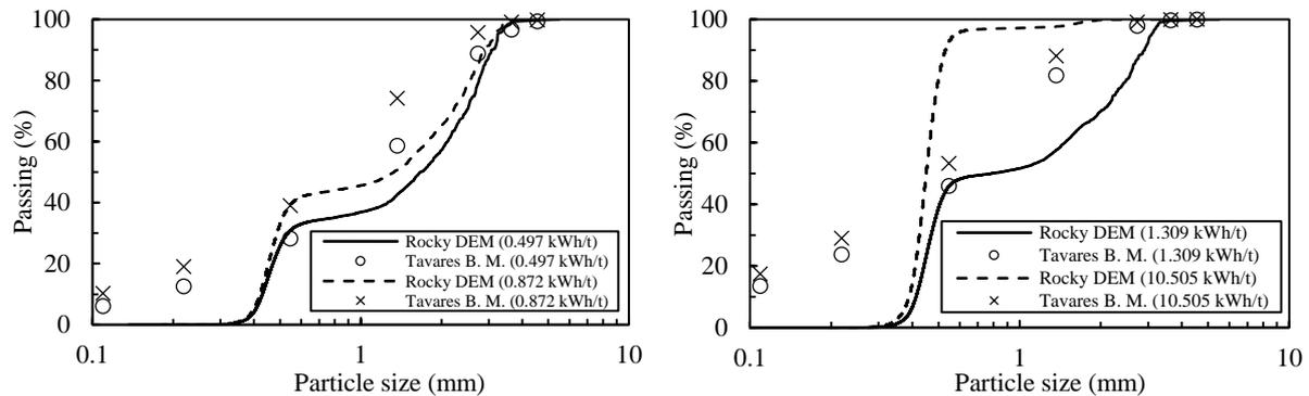
Figure 6 – Comparison between the modelled and simulated progeny size distributions for a single particle impact of particles of 5.47 mm for different impact energies for the limestone particles.
