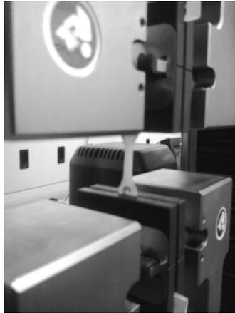
Figure 6: Adhesion tensile test (ASTM 638D, 2002).
