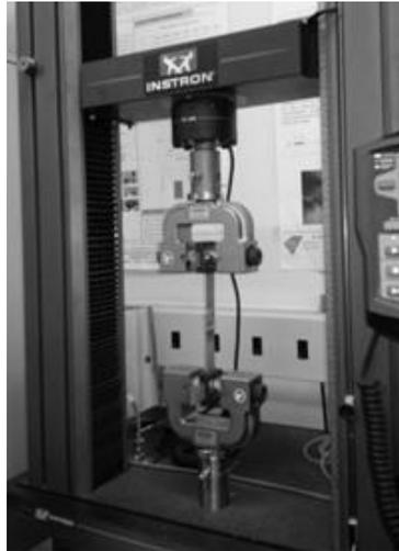
Figure2: Tensile Testing of single shear joints
