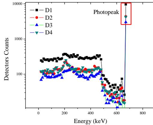
Figure 2 – PHD of four detectors highlighting the photopeak area used to train the ANN.
