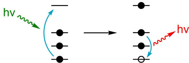
Figure 1- Esquemático representation of X-ray fluorescence.
