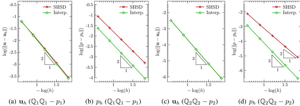
Figure 2-  $h$ -convergence study of the  $\mathbf{u}_h$  and  $p_h$  approximations comparing the hybrid method with the interpolant (Interp.) in  $L^2(\Omega)$  norm for  $\mathbb{Q}_1\mathbb{Q}_1 - p_1$  and  $\mathbb{Q}_2\mathbb{Q}_2 - p_2$  elements.
