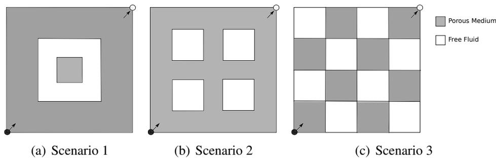
Figure 3- Three coupled porous medium (shaded) free fluid (white) domains used to simulate the five-spot problem.
