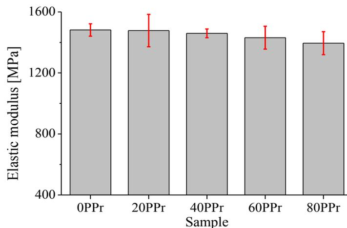
Figure 3- Elastic modulus of PPr/PPv blends.
