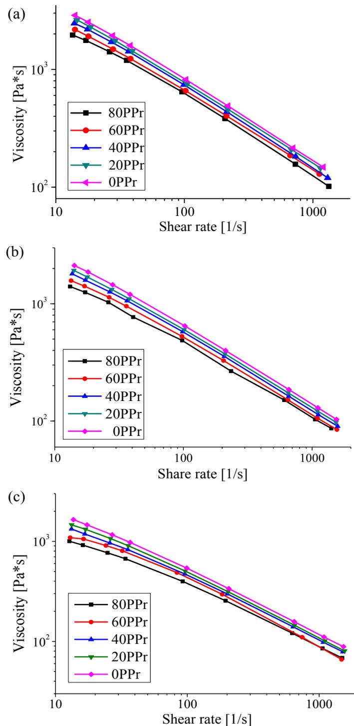
Figure 2- Viscosity of PPr/PPv blends with increasing shear rate at (a) 180°C, (b) 210°C and (c) 240°C.
