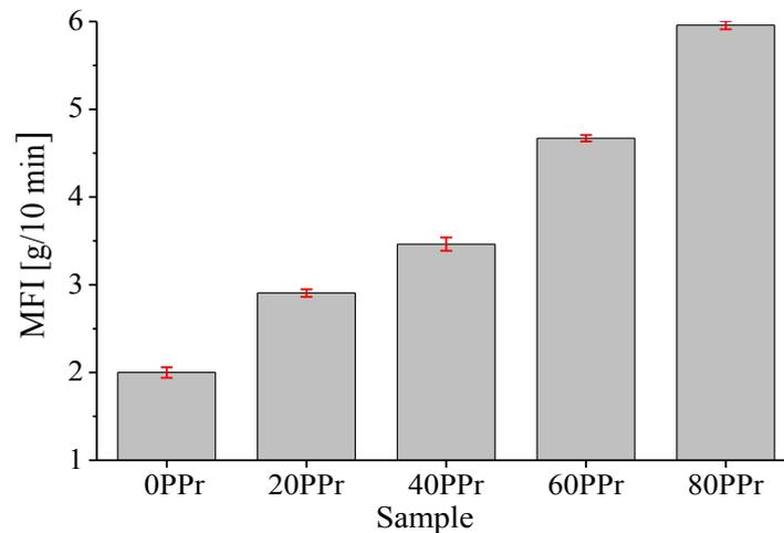
Figure 1- Variation of melt flow index of PPv and PPv/PPr blends.
