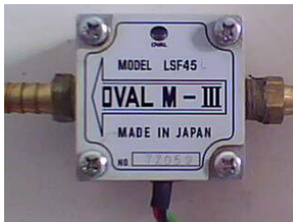
Figure 3. Volumetric sensor to determine the fuel flow
